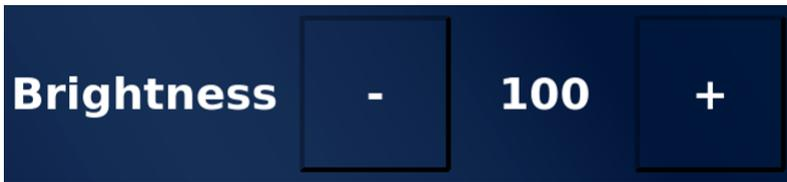
The Brightness buttons regulate the brightness of the device. The brightness can be regulated between 10 and 100 % (of the maximum value).
