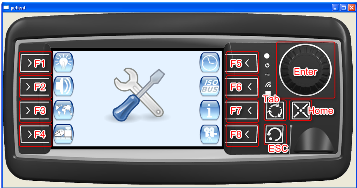
Above: A running PClient simulation on the device with the click areas on the housing marked with red rectangles and the associated keyboard keys.
